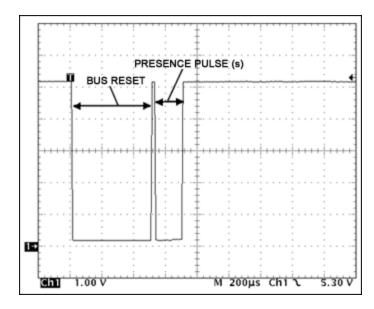
This image also shows a bus reset/presence-detect sequence. The master pulls the bus low for  $480\mu s$ ; all the devices on the bus recognize this as a reset operation. Slaves respond to a bus reset by issuing a presence pulse. Multiple slaves generate their presence pulses during the same period, and the pulses overlap to form a single pulse. (Note that the time base is  $200\mu s$  per division.)
