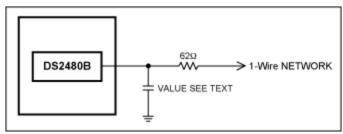
This simple R-C filter improves DS2480B operation on medium-length lines with weights up to 200m. This filter should be used on networks between 10m and 100m when using DS2480B-based master-end interfaces. Depending on the weight of the other components in the network, it is typically recommended to use a capacitor of 470pF. Using a larger value capacitor can add significant load to the DS2480B.
