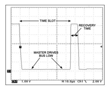
This image shows a Write Zero time slot. The master pulls the bus low for  $60\mu s$  and then releases it for about  $10\mu s$  before another time slot begins.
