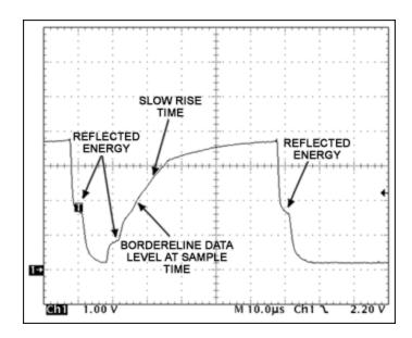
This image shows the effect of excessive weight when using a master with resistor pullup only. The network radius in this example is 300m, and there are 30 devices at the far end of the network. The reflections from the end of the network can be clearly seen, as can the very slow rise time. Note that although this is a Read One time slot, the data level at the sample time is borderline and could be misread by the master.
