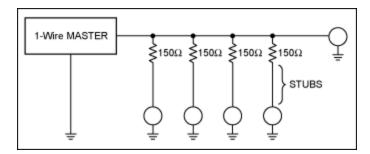
The most successful implementation of this concept uses 150½ resistors at each point where a stub is connected to the main trunk. This value reduces the mismatch at the connection point by about 20%, and attenuates the resulting stub reflections by about 40%. However, the added resistance also degrades noise immunity by about 80%, so caution must be observed. Tests have also shown good performance using 100½ resistor values, which do not degrade noise immunity quite as much.
