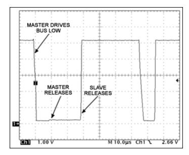
This image shows a Read Zero time slot. The master pulls the bus low for about  $10\mu s$  and then releases it. However, a slave is returning a zero bit by holding the bus low for a longer time. The slave's time base can vary between  $15\mu s$  and  $60\mu s$ .
