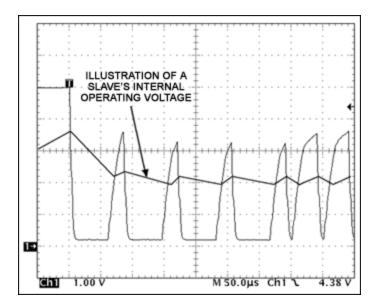
When rise time is slow, the recovery time (the period between time slots) may not be long enough to allow the bus to reach a voltage level sufficient to recharge the slaves. In the image above, the slave's
