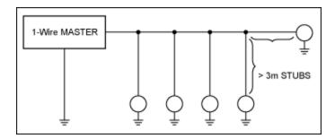
3. Star topology: The 1-Wire bus is split at or near the master end and extends in multiple branches of varying lengths. There are slave devices along, or at the ends of, the branches.
