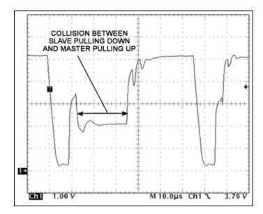
This image shows the resulting chaos that occurs when the active pullup is falsely triggered by reflections on the cable due to stubs and branches. This is a Read Zero time slot, although the reflection has caused the active pullup to activate and collide with the pulldown in the slave device.
