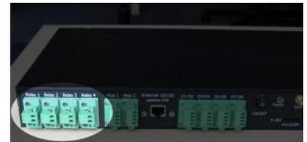
The relay outputs on the front panel
